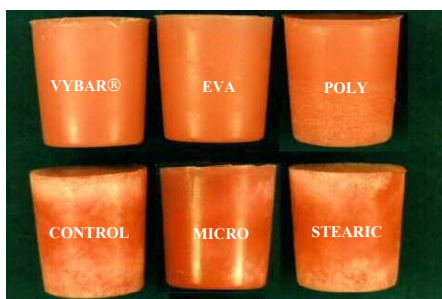
Figure 4: The effect of various chemical additives at 0.25% (w/w) on mottling: a) Vybar ® b) EVA c) Polyethylene d) Control e) Microcrystalline wax f) Stearic acid
