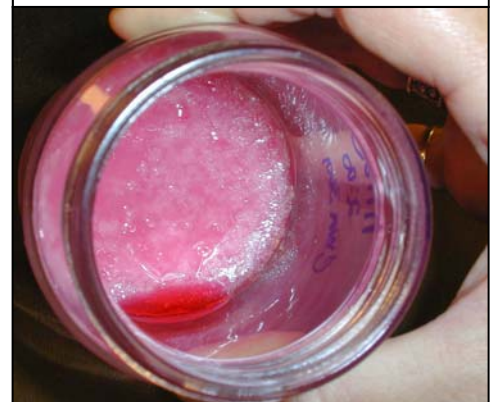
Figure 1: Evidence of Syneresis in a Container Candle
