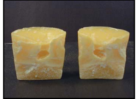
Figure 3: Cross-section of a votive candle showing brittleness
